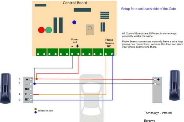
The best install height should be around 500mm from the ground, the distance between each senor should be no more then 15m. This model YET609 can except 12 to 24V DC/AC power.
