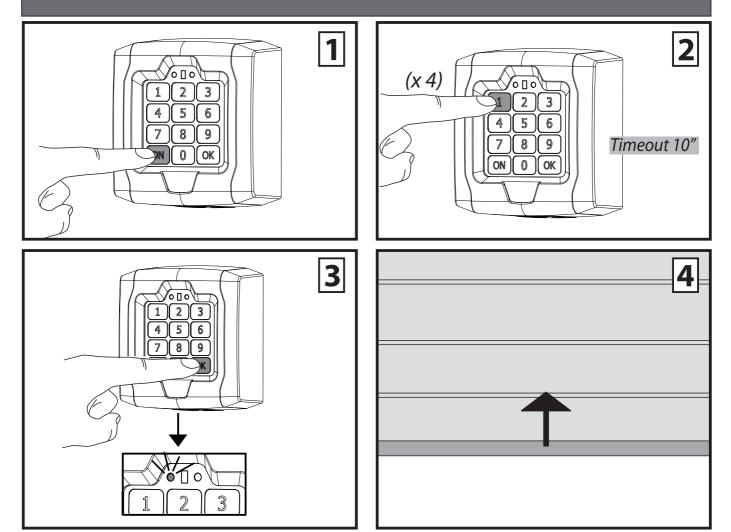
**WARNING:** Q.BO TOUCH will lockout after 3 consecutive incorrect codes are entered and will not accept further codes for 90 seconds. If another incorrect code is entered, Q.BO TOUCH will lockout at the first attempt.
