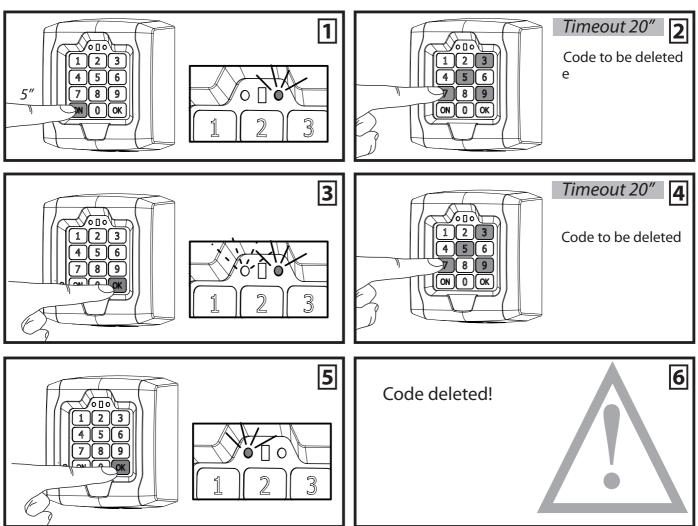
**WARNING:** if you delete the last code, you will no longer be able to activate the relevant control unit. To restore operation, you must perform the total deletion procedure to erase all codes and repeat installation from the beginning. It is advisable to delete the codes of channels that are not associated with anything (e.g. code 2222, 3333, 4444, 0000 etc. when using a single control unit).
