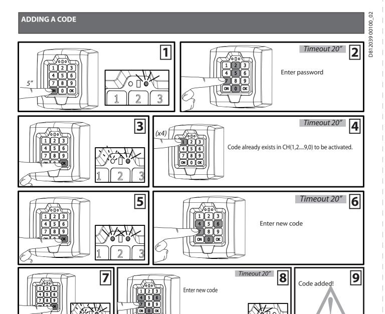
**WARNING:** To add a code, you need to know the system password. Q.BO TOUCH can handle up to 100 different codes. The new code will serve the same purpose as the existing code (activates the same channel).
