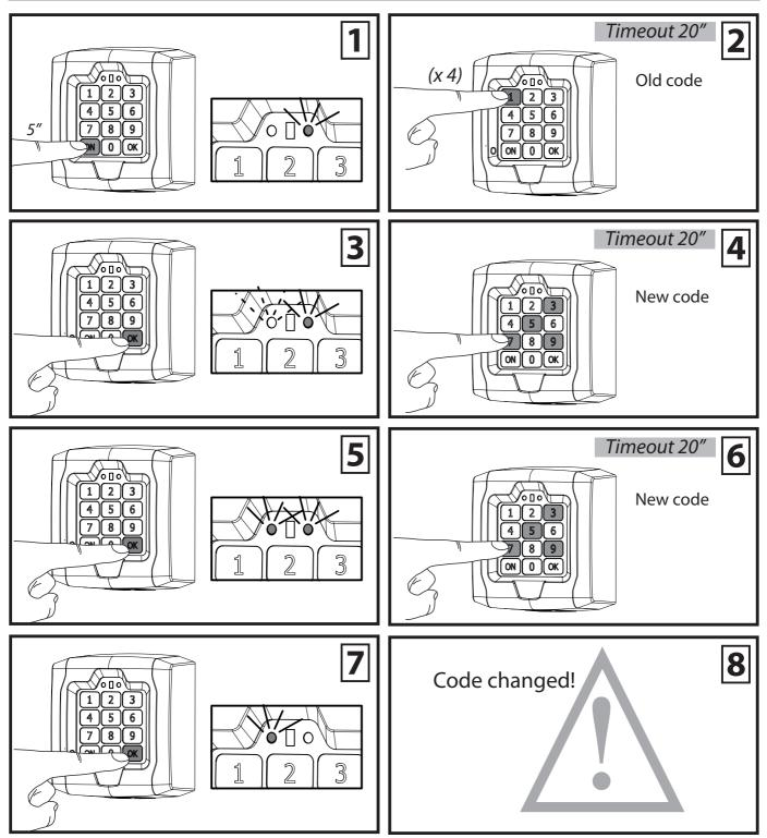
**WARNING:** the code consists of a sequence of no less than 4 and no more than 7 digits (in the range 0 to 9). Do not use codes with all the same numbers. (e.g. codes like 2222, 3333, 4444, 0000 etc.).
