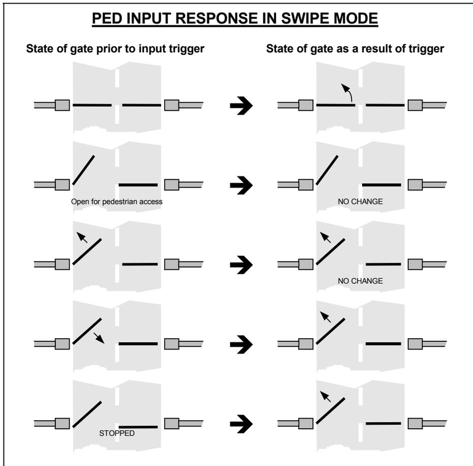
Figure 13 PED Input Response In SWIPE Mode
