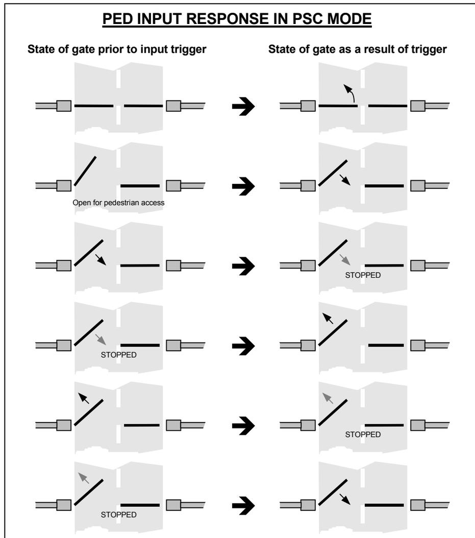
Figure 12 PED Input Response In PSC Mode
