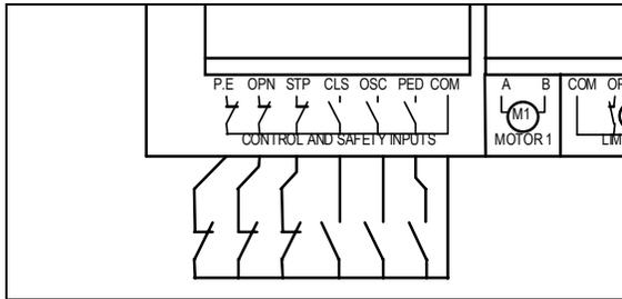
**AT NO TIME SHOULD A VOLTAGE OR CURRENT BE APPLIED TO THE INPUTS AS THIS MAY PERMANENTLY DAMAGE THE CONTROL BOARD OR SEVERELY REDUCE ITS RELIABILITY. SWITCH WIRING SHOULD BE KEPT AS SHORT AS POSSIBLE AND AWAY FROM SOURCES OF ELECTRICAL INTERFERENCE AS THIS MAY FALSELY TRIGGER THE CONTROL BOARD'S INPUTS.**
