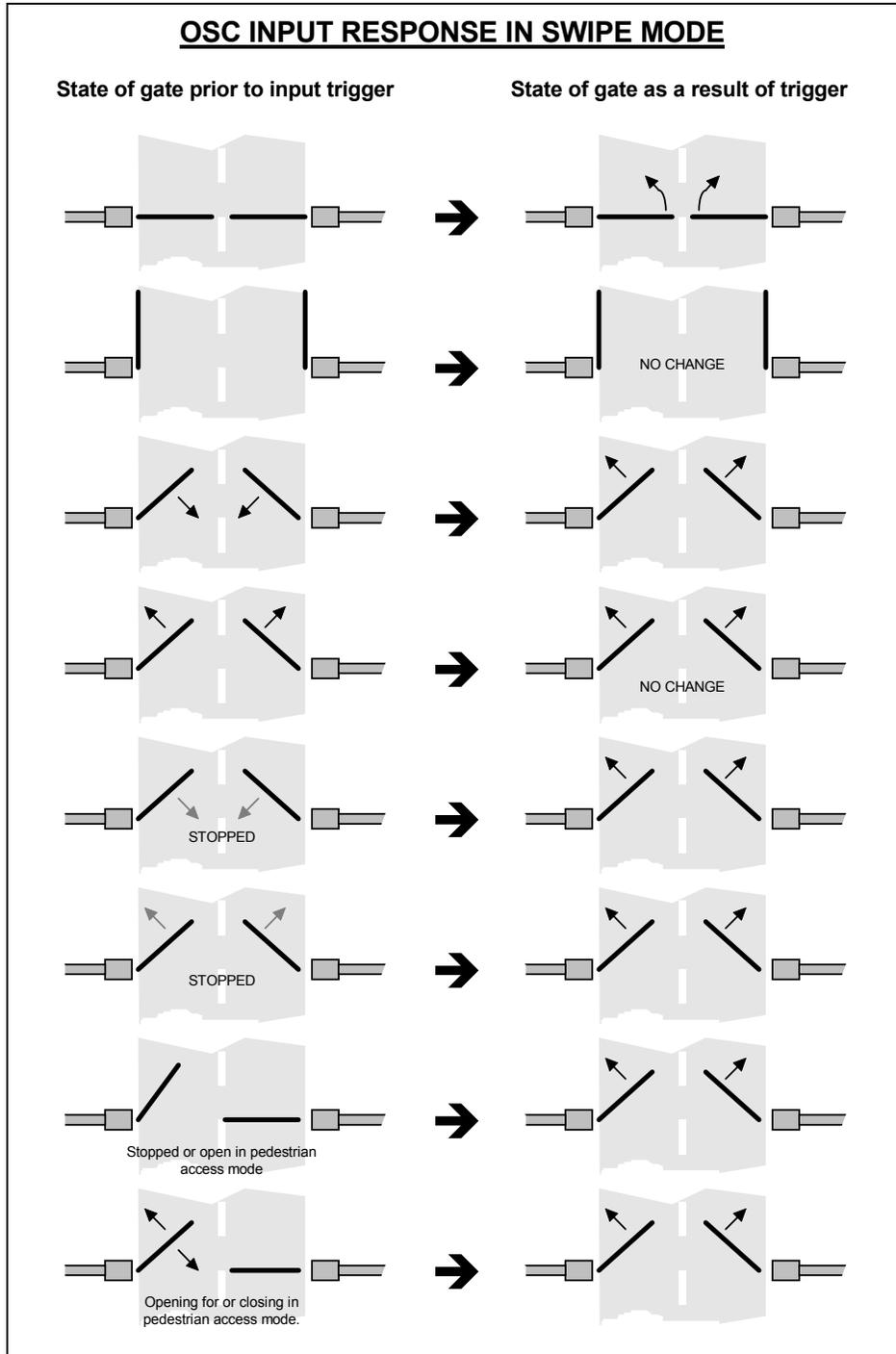
Figure 11 OSC Input Response In SWIPE Mode
