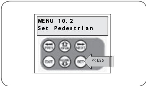
**NOTE:** Before setting the pedestrian access position the gate must be in the fully closed position. As with the Setting Travel Limit procedure, a transmitter can be used to complete the pedestrian position setting procedure.
