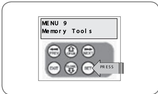
The Memory Tools accessed from within Menu 9 are used to backup, restore or clear the controller's memory. Once selected the PREV or NEXT buttons can be used to view the Memory Tool options. To Execute the displayed option simply press SET.
